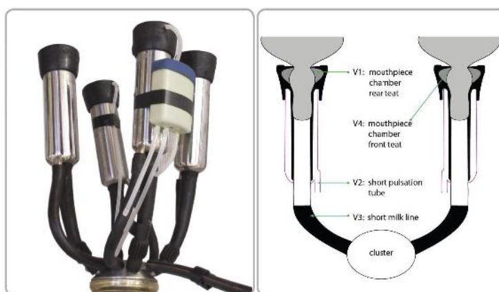
VaDia data logger records the vacuum at 4 points in the milking cluster
